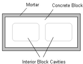
**Figure 1: Construction of Typical Concrete Block**
